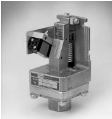
Open pneumatic pressure switch assembly. Five ported four way valve is actuated by transducer mechanical displacement when pressure exceeds adjustable set point. Shown with optional barb connectors installed.
