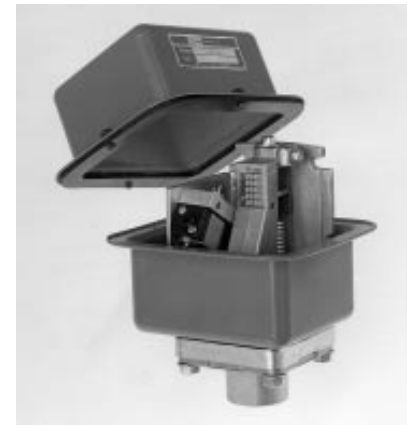
Pneumatic pressure switch has gasketed enclosure. Adjusting nut sets pressure at which pneumatic valve is actuated. Shown with optional barb connectors installed.
